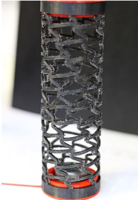
Fig. 9. Large deformation of ligaments under tensile load, at 42% strain.
